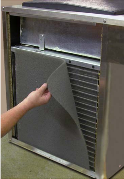
Figure 3-11 F112 Condenser Filter Removal
